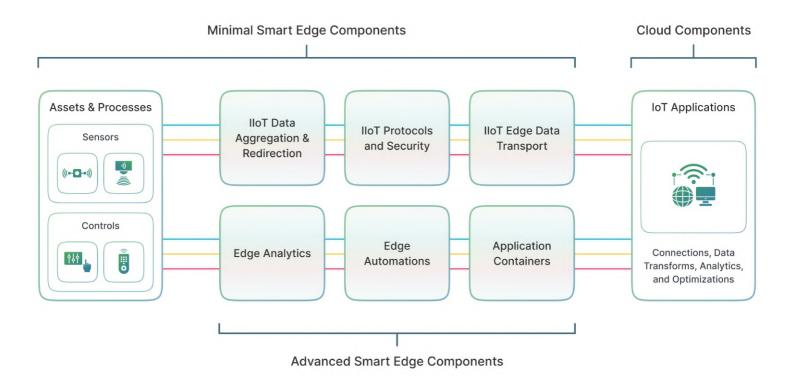
While building edge IIoT solutions is well understood from a technology and engineering perspective, until recently building edge IIoT intelligence has been a somewhat involved process. Identifying and integrating the appropriate sensors, selecting a suitable CPU and connectivity architecture, building a secure embedded processing engine, and managing secure connections to whatever cloud IIoT Platform services used required significant investment and expertise.
